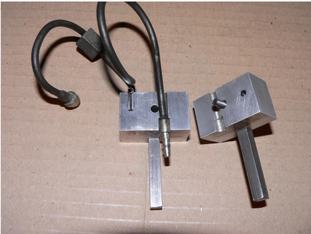
8. Squeeze the two halves of the top section together, clamping the barb or banjo between them. Then slip the alignment pins into the square grooves along the bottom section. The vice jaws holding the bottom half will also hold the top section together by the square alignment pins.
